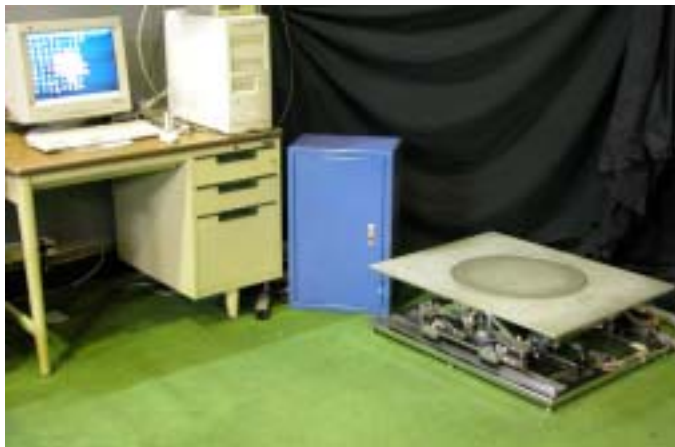
Fig. 1 Triaxial Postural Perturbation Platform
