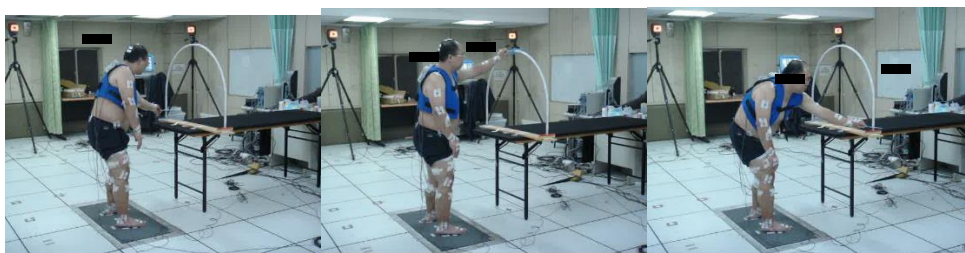
Figure 1. Experiment setup of the motion analysis with a single curved shoulder arc for stroke patient
